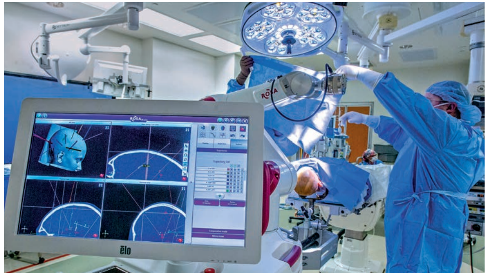
ROSA One Brain is used in the OR to guide surgical instruments into place based on the surgery plan created prior to entering the OR. This guidance means less time in the OR, more electrodes that can be placed and a higher chance of finding seizure locations.
